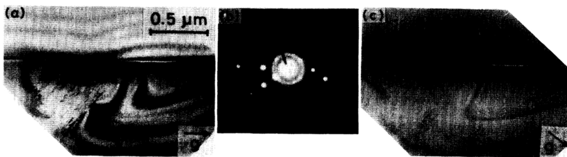
Fig. 28. Cross-sectional TEM images of the damaged zone by scratching (a) diffraction vectors g [220] and (c) g [222] . (b) SADP of the damaged zone [79].
